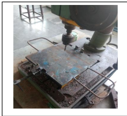
Fig.8. Drilling of mild steel plate
